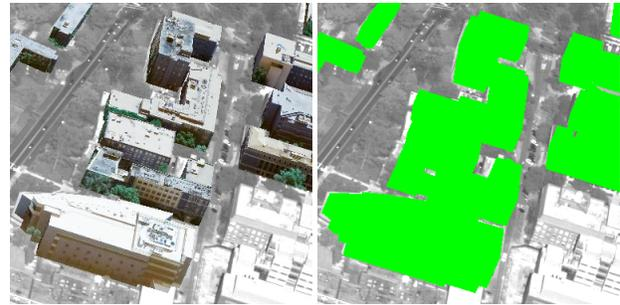
Figure 3. Example of the accuracy of the camera pose estimation. Accurate estimate of the camera pose results in a good registration of the 3D models (left) and occlusion map (right) with the image sequence.
