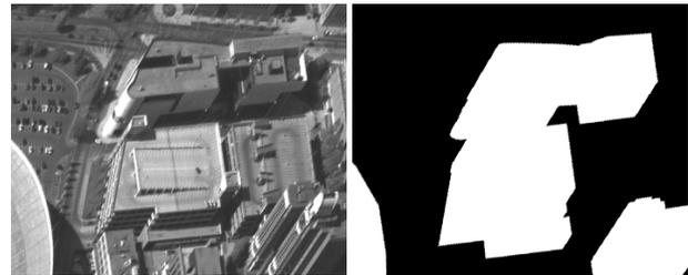
Figure 1. Automatically computed occlusion map (right) for the image on the left.
