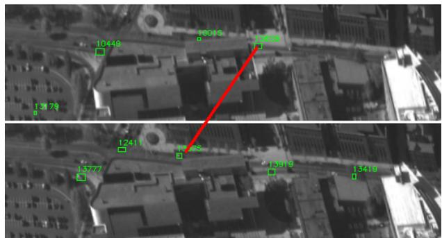
Figure 8. Another example of a linked track by the proposed algorithm. The top row shows the vehicle before occlusion and the bottom row shows the same vehicle after occlusion.
