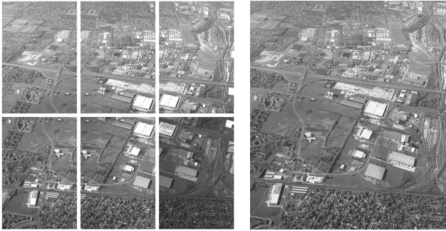
Figure 1. One frame of the imagery is captured by an array of cameras (left), while it is desirable to work with only one image per frame, as if it were captured by a virtual camera (right).
